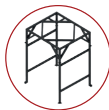
Discharge structure in Big-Bag (optional)
