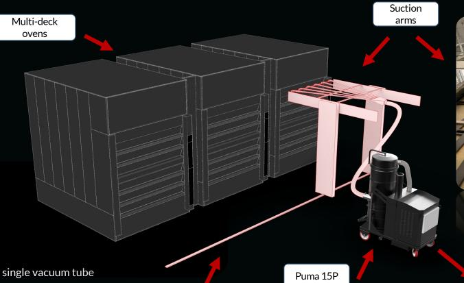
Rail which allows the structure to move horizontally
