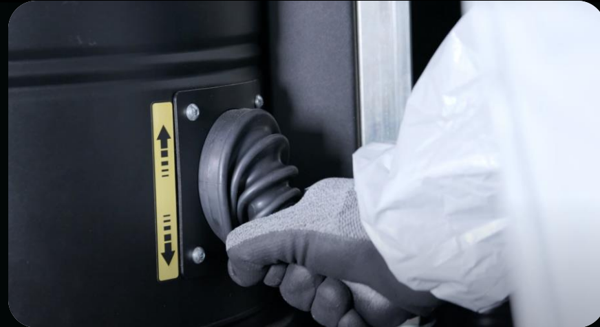
Manual filter cleaning system
